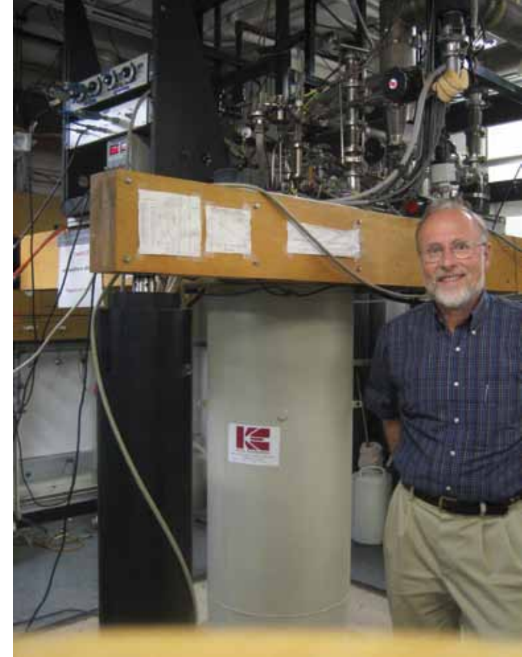
Bill Halperin and the ultra-low temperature demagnetization cryostat. This cryostat requires the rare isotope, helium-3, to achieve temperatures less than one thousandth of a degree from absolute zero temperature. Photo by Jai Li.
